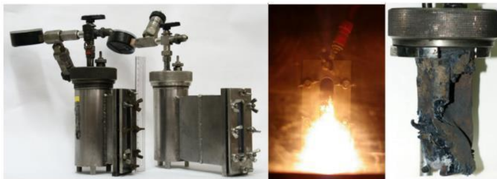
Fig. 2. The experimental set-up for SHS (left), the light signal emitted during combustion as an observation via polycarbonate window (middle), and raw sponge-like product (right).
