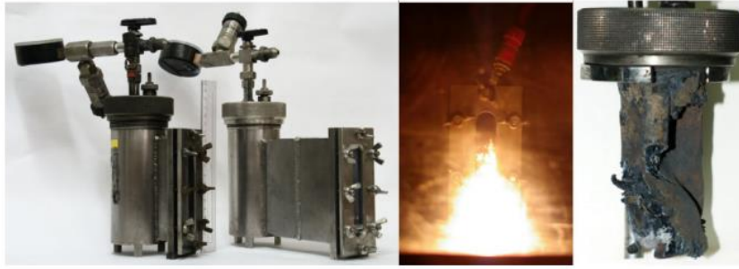
Figure 7-4 The experimental set-up for SHS - left, the light signal emitted during combustion as an observation via polycarbonate window - middle, and raw sponge-like product – right (Copyright © 2013 WILEY-VCH Verlag GmbH & Co. KGaA, Weinheim) [37].
