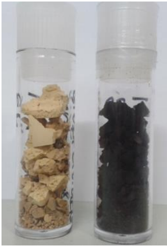
Figure 7-1 Intermediate dried samples of SiO 2 -citric acid xerogels: SiC_1 (right) and SiC_2 (left).
